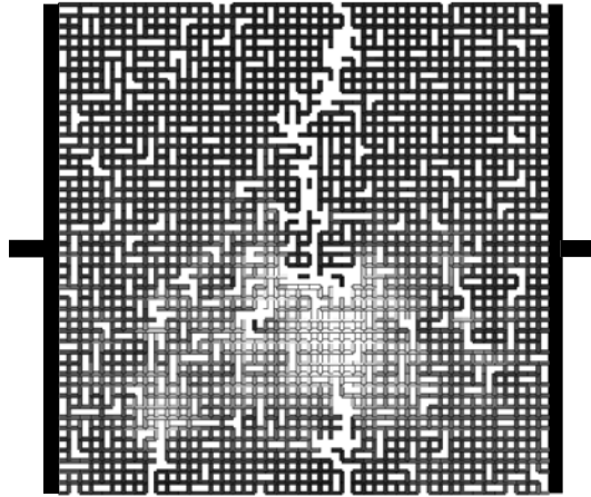
Figure 1. Network evolution near the electrical breakdown. Different grey levels from black to white correspond to increasing values of r_n from 1 to 3 ( \Omega ).
